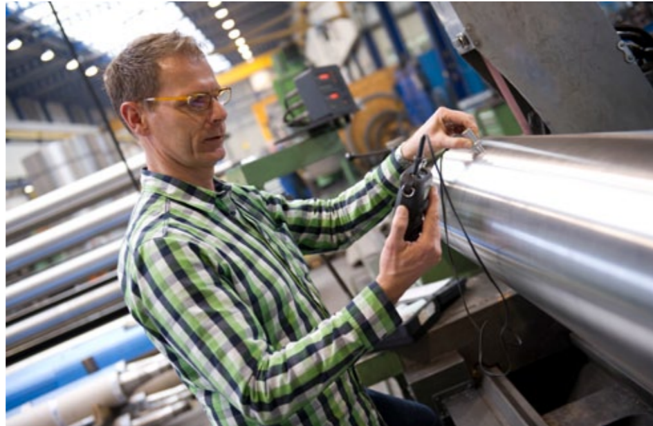
▲ Wall thickness measurement
