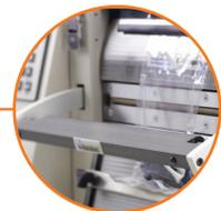
Open load area and controlled seal bar maximise loading flexibility and operator safety
