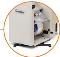
Locking turntable and AutoThread™ feature provide easy bag access and changeover
