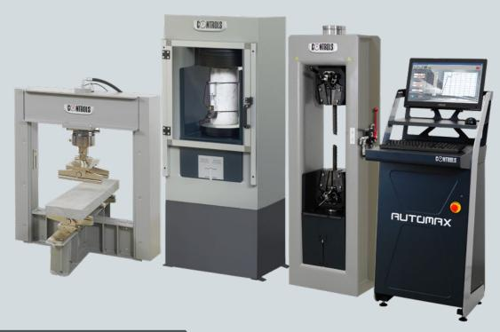
Rev-up your testing system with additional frames, accessories and dedicated software packages to perform many tests including compression, flexural, cyclic modulus of elasticity and Poisson's Ratio, steel tensile tests and more.
