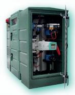
Guillotine integrated in Heavy Duty Effluent Control station.
