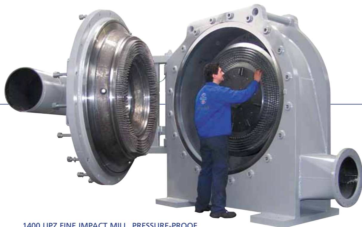
1400 UPZ FINE IMPACT MILL, PRESSURE-PROOF TO 0.3 BAR OVERPRESSURE, GAS-TIGHT
